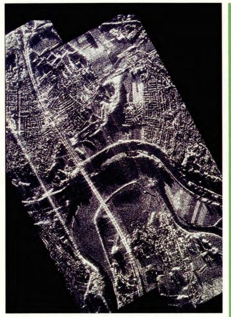
No bridge too far: The Rhine River and the surrounding countryside is clearly shown winding its way through Germany in this picture of the Joint STARS Synthetic Aperture Radar (SAR) mode. This mode furnishes imagery of land features, along with mobile targets that have become stationary, providing CSAR-dedicated forces with details concerning the terrain where downed crewmembers may be located.
