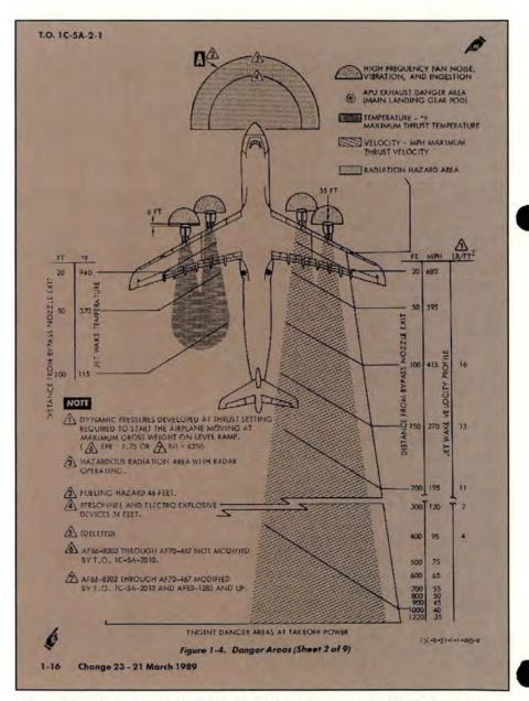
This graphic taken from Technical Order 1C-5A-2-1 provides a visual representation of the velocity of the blast from the C-5 engines.
