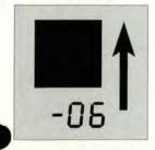
A solid red square indicates that the intruding aircraft is projected to be a collision threat. TCAS II calculates that the intruder has reached the point where a resolution advisory is necessary. The time to closest approach with the intruder is now between 20 and 30 sec-
